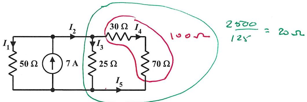
Use equivalent resistance and the current divider equation to determine each of the following:
